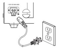
**Caution:** The supplied power cord has a polarized plug that fits into the outlet only one way. If the plug does not fit properly, turn it over and try again. Do not force it.
